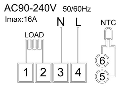
LOAD – connected device N, L – thermostat's power supply NTC – floor sensor
